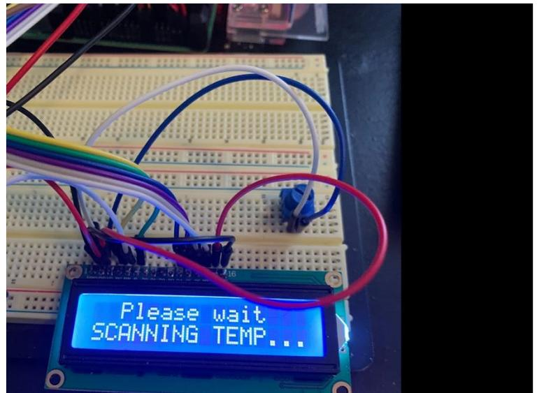
Figure 22: 16x2 Character LCD Screen Testing [15]
